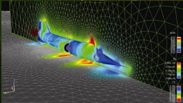
This digital rendering of the NAE is used to run CFD analysis whereby different nose cone, canard and wheel fairing designs are evaluated.
